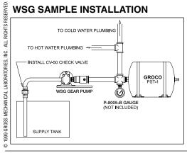
**Start-up:** Double-check plumbing connections. Pour a small amount of water into the inlet hose to aid in initial prime. Open all faucets and showers and apply power. When the pump primes and a smooth water flow comes from each outlet, shut it off. When all outlets are closed, the pump will fill the water heater and PST-1 tank (this may take a few minutes) and shut off at 38-40 PSI. Check once again for leaks.
