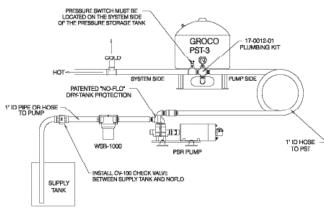
**PLUMBING:** Fasten 17-0012-01 plumbing kit onto the PST (pressure storage tank) with the pressure switch on the system-side of the PST and the hose barb on the pump-side of the PST as shown above. To aid in initial priming, pour water into the pump inlet before connecting hoses to the pump. Plumbing between the pump and the PST must be 1" ID heavily reinforced hose, and must be free of valves, filters, or any other device. Plumbing after the PST may be reduced.
