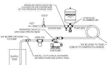
**PLUMBING:** Fasten 17-0012-00 plumbing kit onto the PST (pressure storage tank) with the pressure switch on the system-side of the PST and the hose barb on the pump-side of the PST as shown above. To aid in initial priming, pour water into the pump inlet before connecting hoses to the pump. Plumbing between the pump and the PST must be 3/4" ID heavily reinforced hose, and must be free of valves, filters, or any other device. Plumbing after the PST may be reduced.
