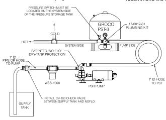
Mount the pump to a sturdy platform using the four (4) mount feet included. Operation will be quieter if mounted to a solid surface.
